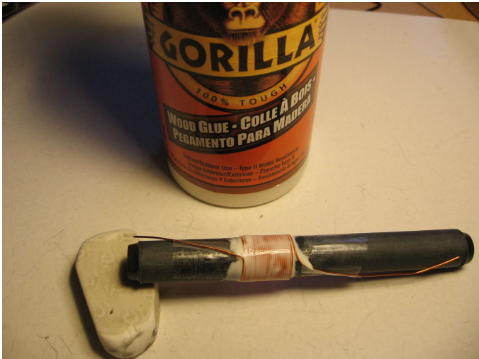
Figure 18 Winding antenna coils
