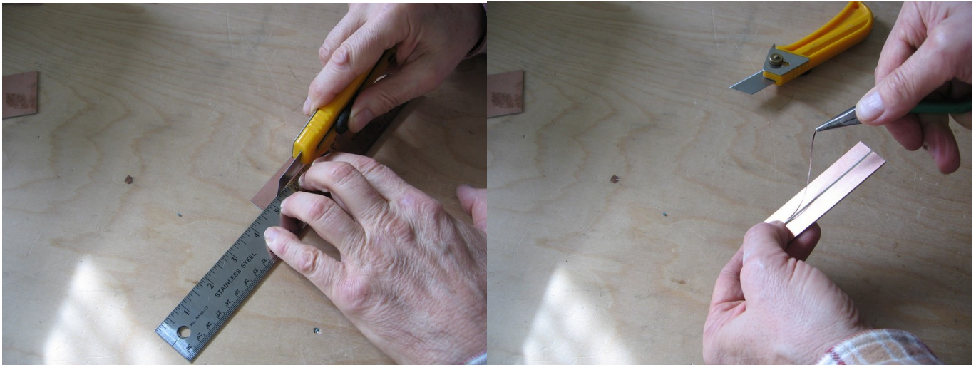
Figure 3. Preparing the antenna mounting box/shield
